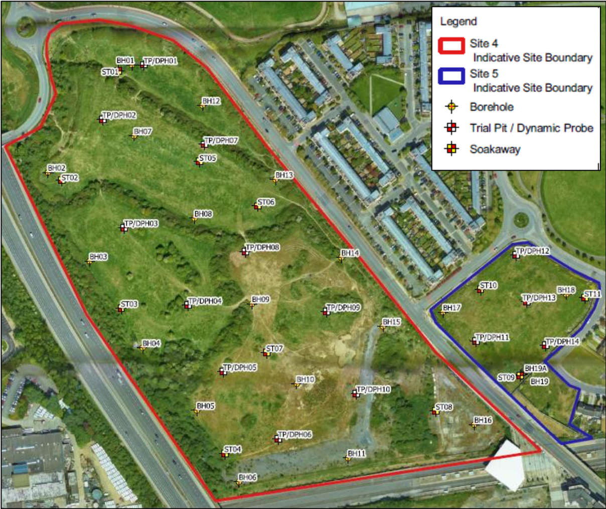
Figure 2 | Site Investigation Test Locations
